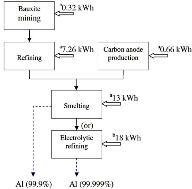
Figure 2 Total energy requirement of primary Al production[3]
