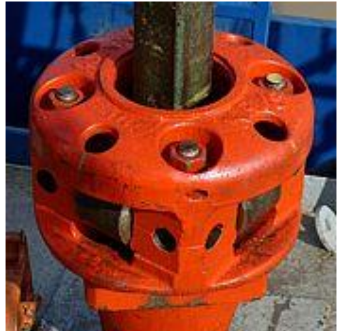
Kelly fitted into drive bushing
